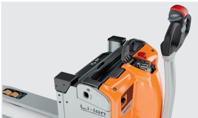
Excellent availability thanks to integrated quick-charging access for flexible and efficient charging and intermediate charging of the lithium-ion battery
